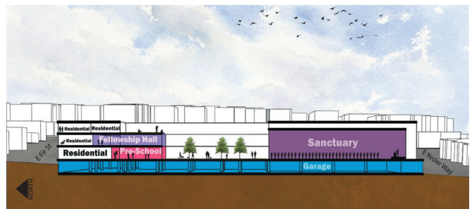
Early proposal building section facing east along 15th Ave showing courtyard relationship to surrounding uses
