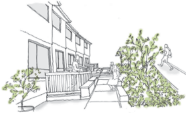
“Residential units provided with individual, private outdoor spaces, a shared, semi-public walk with seating, and landscape buffer next to the public sidewalk.” SCHEMATA WORKSHOP, CANDG
