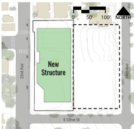
Proposed site plan shows one shared building on the west half of site, allowing potential sale or separate development of open eastern half.
